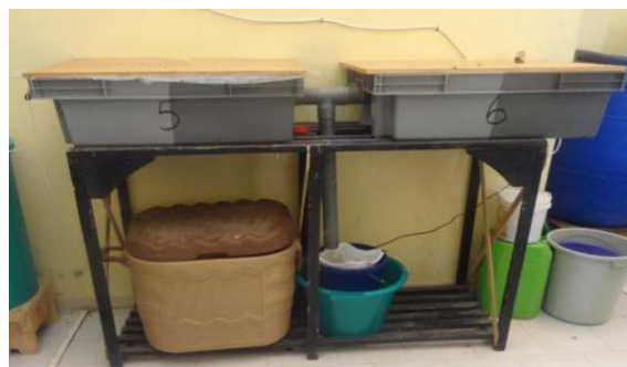
Figure 4: Tanks 5 and 6 of genitors were connected to a biofilter (bucket under desk).
