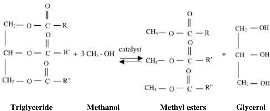
**Figure 1:** The overall chemical reaction of the transesterification process.
