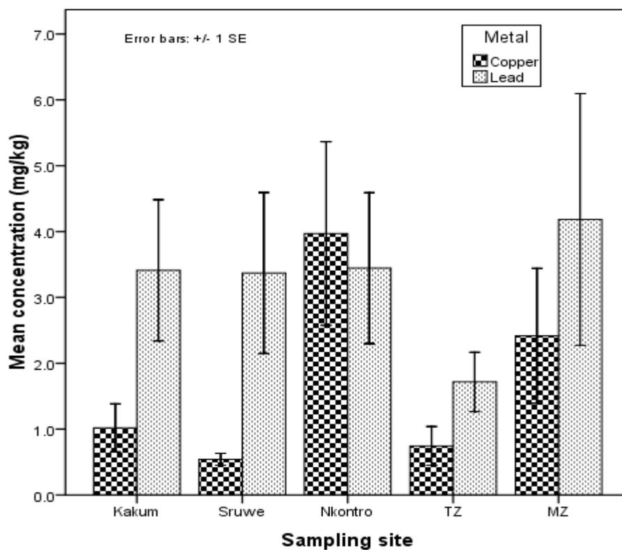
Figure 2: Variation of Cu and Pb concentrations in leachate sediment samples from sampling sites.
