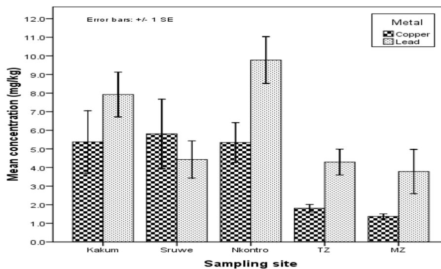
Figure 3: Variation of Cu and Pb concentrations in residue sediment samples from sampling sites.
