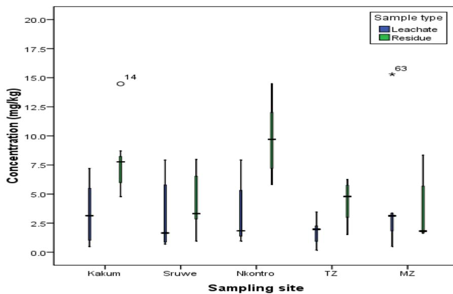
Figure 5: Box plot for lead concentrations in leachate and residue sediment samples.
