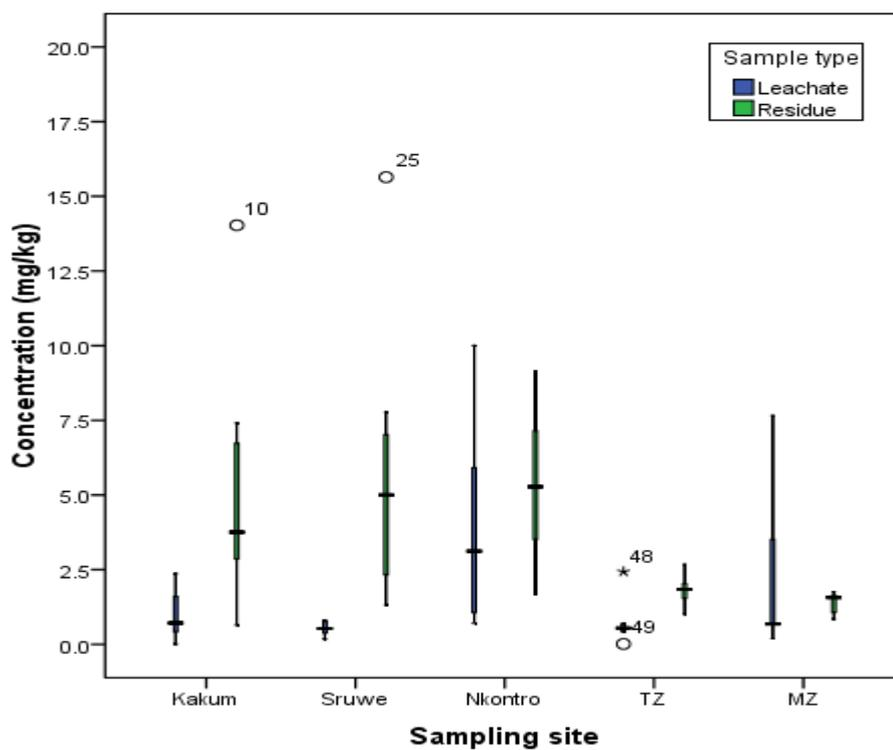
Figure 4: Box plot for copper concentrations in leachate and residue sediment samples.
