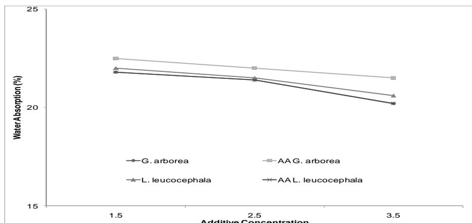
**Figure 4:** Water absorption of boards using different additive concentration.
