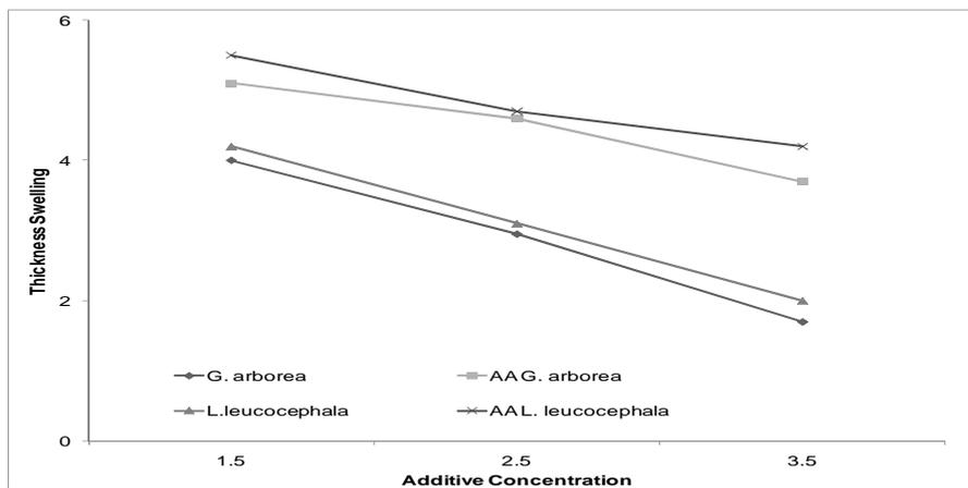
Figure 3: Thickness swelling of boards using different additive concentration.
