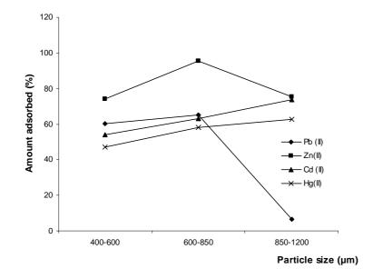
**Figure 4:** Percent adsorbed % against particle size ( $\mu$ m) for adsorption of Pb (II), Zn (II), Cd (II), and Hg (II) onto modified broad leafed pompkin pods (MBLPP).
