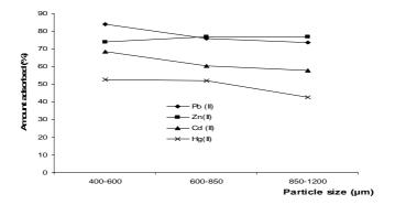
**Figure 2:** Percent adsorbed % against particle size ( $\mu$ m) for adsorption of Pb (II), Zn (II), Cd (II), and Hg (II) onto unmodified broad leafed pompkin pods (UBLPP).
