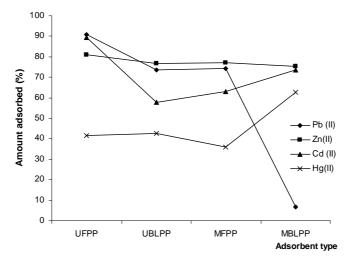
**Figure 6:** Percent adsorbed % for adsorption of Pb (II), Zn (II), Cd (II), and Hg (II) onto the different adsorbent types for particle size of  $850-1200 \,\mu$ m.
