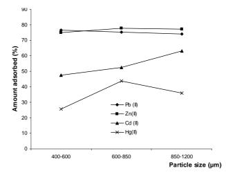
**Figure 3:** Percent adsorbed % against particle size ( $\mu$ m) for adsorption of Pb (II), Zn (II), Cd (II), and Hg (II) onto modified fluted pompkin pods (MFPP).
