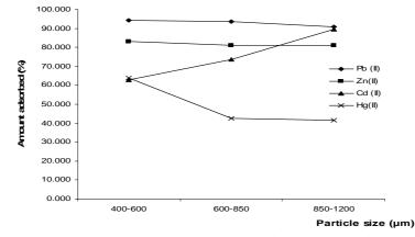
**Figure 1:** Percent adsorbed % against particle size ( $\mu$ m) for adsorption of Pb (II), Zn (II), Cd (II), and Hg (II) onto unmodified fluted pompkin pods (UFPP).
