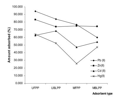
**Figure 5:** Percent adsorbed % for adsorption of Pb (II), Zn (II), Cd (II), and Hg (II) onto the different adsorbent types for particle size of 400-600  $\mu$ m.
