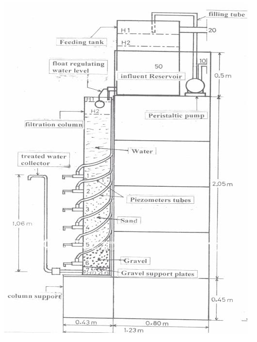
Figure 1: Schematic of pilot plan used in slow sand filtration.
