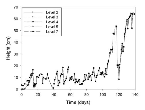
Figure 2: Evolution of head losses at different levels of the column.
