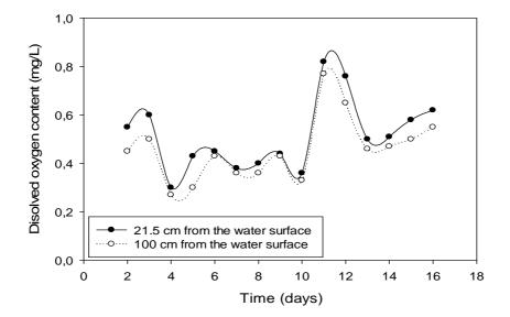
Figure 3: Changes in oxygen content in the filter close to the primary settling tank.
