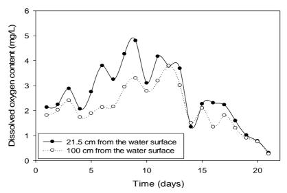
Figure 4: Variation in the oxygen content in the filter placed near the clarifier.
