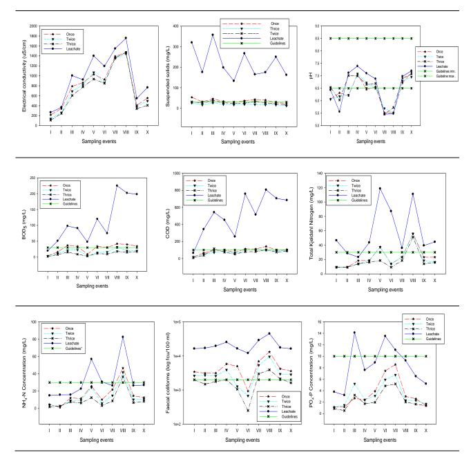
Figure 3: Characteristics of the effluents after treatment in CVFCW following one, two or three applications daily.
