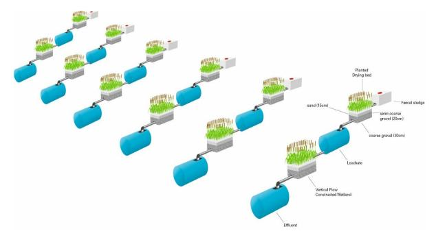
**Figure 1:** Schematic of the University of Yaoundé I pilot-scale faecal sludge treatment plant facility including how terminology is defined in this paper.
