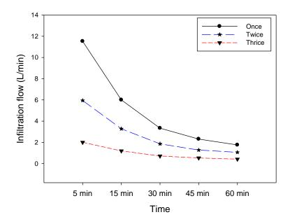
Figure 2: Infiltration flow rate as function of time and feeding frequencies.
