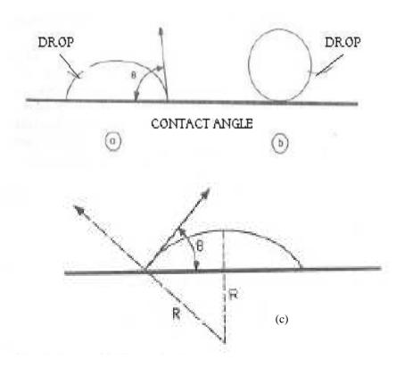
Figure 1: (a) Contact angle  $\theta$  of a drop that wets the solid surface. (b) Contact angle (180°) of a drop that does not wet the solid surface. (c) Determination of contact angle of a drop of radius R on a solid surface.
