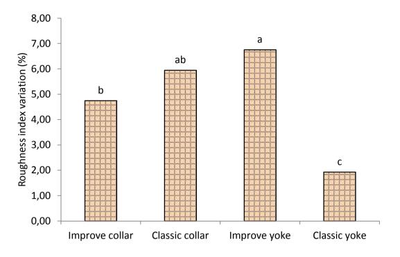
**Figure 6**: Soil roughness index variation after the tillage. N and K test: a, ab, b, c, are groups of means significantly different at  $\alpha = 0.05$  level.
