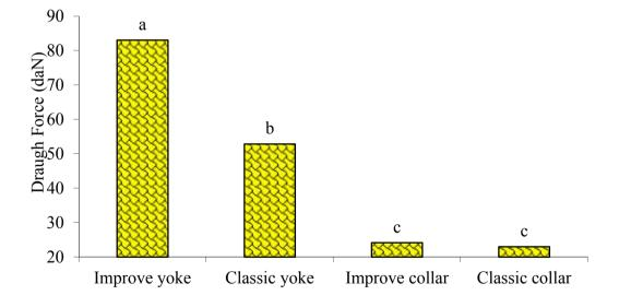
Figure 5: Traction force variation according the type of harnessing. N and K test: a, b, c, are groups of means significantly different at  $\alpha = 0.05$  level.
