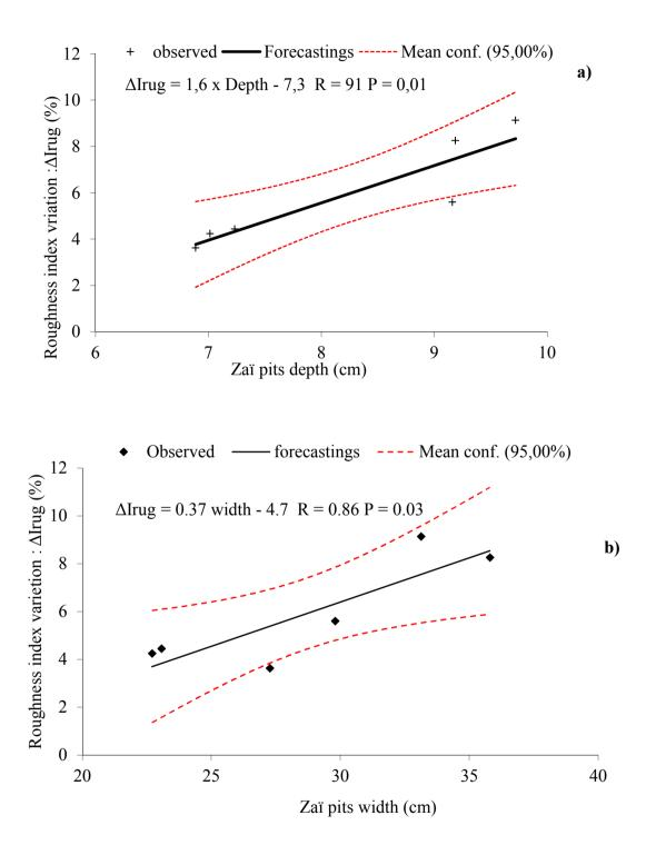
**Figure 7**: Roughness increase according to the pits depth (a); Roughness increase according to the pit width (b).  $\Delta$ Irug: roughness index variation, R: regression coefficient, P: probability.
