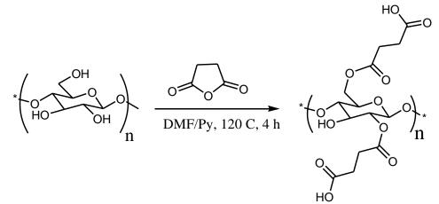
**Figure 1**: Esterification of hardwood cellulose fibers by succinic anhydride molecule in N,N-dimethylformamide (DMF) and pyridine (Py) at 120 °C for 4 hours.
