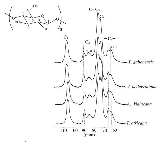
**Figure 5:** <sup>13</sup>C CP/MAS NMR spectra of unesterified tropical hardwood cellulose fibers. (i): chains of crystal interior cellulose. (s+a): chains exposed on crystal surface plus amorphous cellulose.
