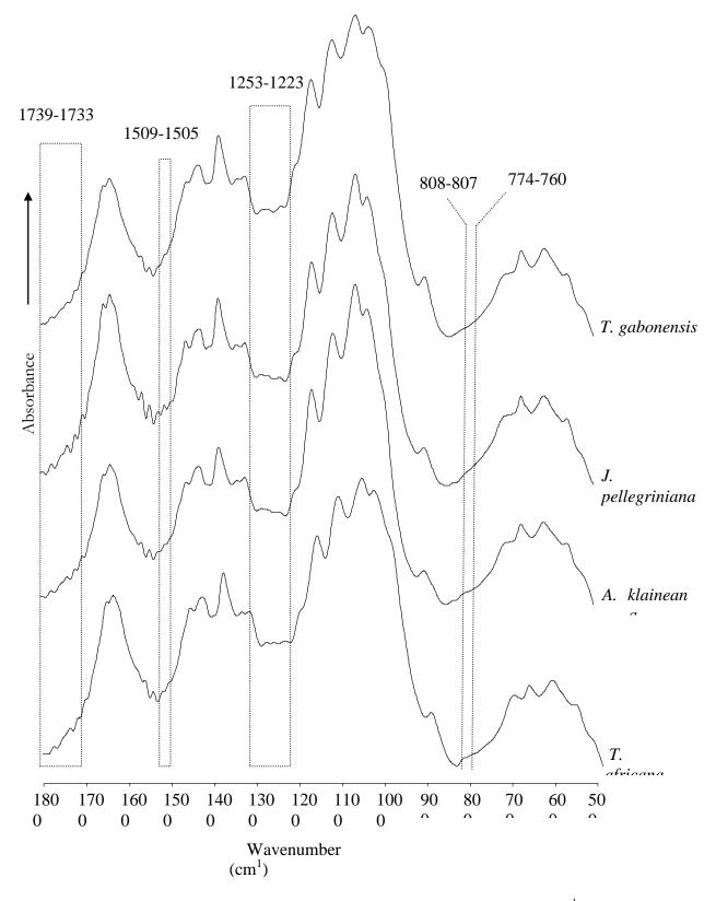
Figure 3: FTIR spectra of tropical hardwood cellulose fibers in the range 1800-500 cm<sup>-1</sup>.
