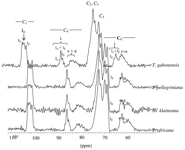
**Figure 6:** In the top, a portion of baseline corrected and deconvoluted spectra of the C-4 region of signals assigned to the interior chains of unesterified *T. gabonensis* (a), *J. pellegriniana* (b), *A. klaineana* (c) and *T. africana* (d) cellulose fibers respectively, derived from the spectra enhanced (bottom). (i): chains of crystal interior cellulose chains. (s+a): chains exposed on crystal surfaces plus amorphous cellulose. ( $\blacklozenge$ ): Noise.
