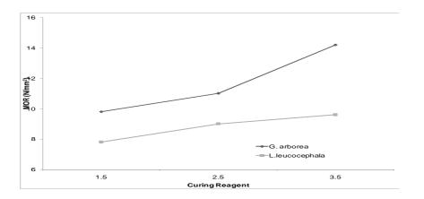
Figure 2: MOR of boards with G. arborea and L. leucocephala using different curing reagents.
