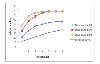
Figure 1: The graph of % moisture loss from waterleaf subjected to different heat treatments and drying methods.
