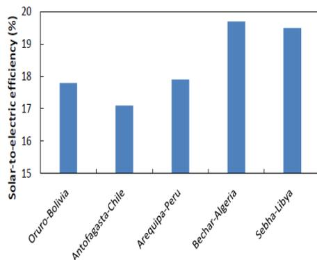
Figure 5. Solar-to-electric efficiency of HSGT
