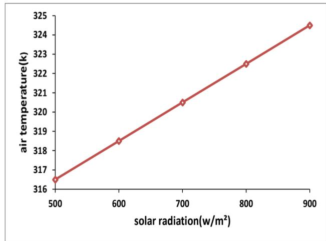
Figure 7. Effect of solar radiation on temperature
