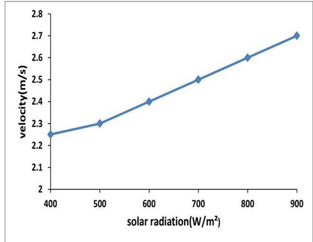
Figure 6. Effect of solar radiation on air velocity
