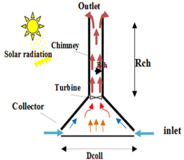
Figure 1. diagram Schematic of solar chimney power plant
