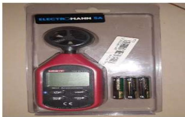
Figure. 2. UT363 Wind Anemometer
