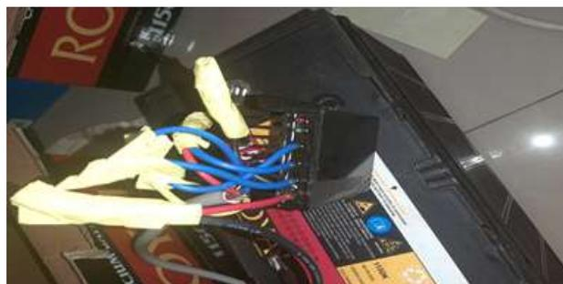
Figure. 6. Charge controller connected to the batteries during testing in Soweto.
