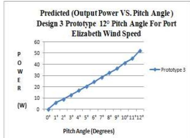
Figure 16. Predicted (output power vs. blade maximum pitch angle as derived for Prototype 3 in Gqeberha (PE) region).
