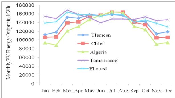
Figure 10. PV electrical energy production for studied areas using Si-crystalline
