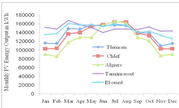
Figure 9. PV electrical energy production for studied areas using CIS technology.
