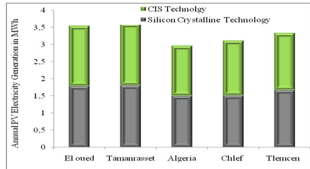
Figure 11. Annual PV energy output for selected areas using Si-crystalline and CIS technology
