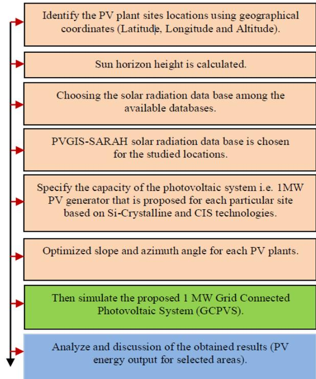
Figure 7. Simulation methodology of 1MW grid connected PV system
