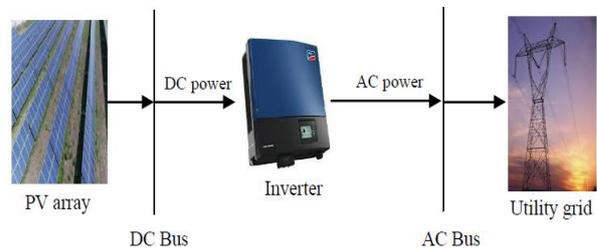
Figure 5. PV Grid connected system scheme
