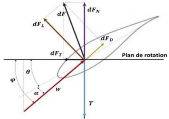
Figure 1. Flow effect on blade section [5].
