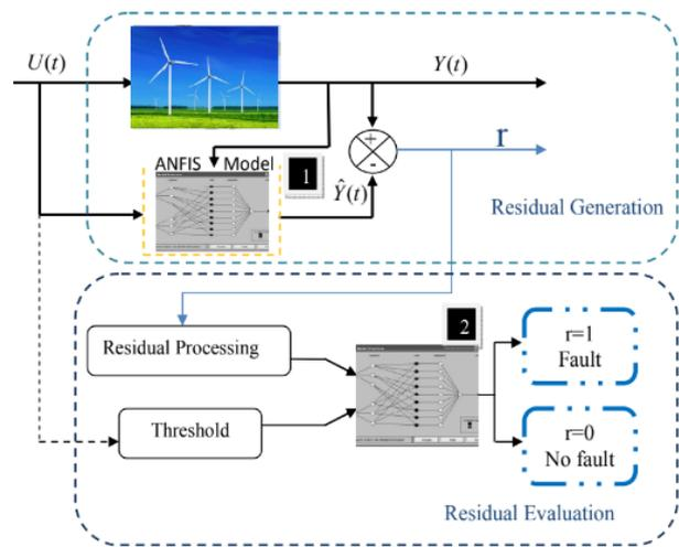
Figure 3. Structure of the diagnosis approach based on ANFIS models
