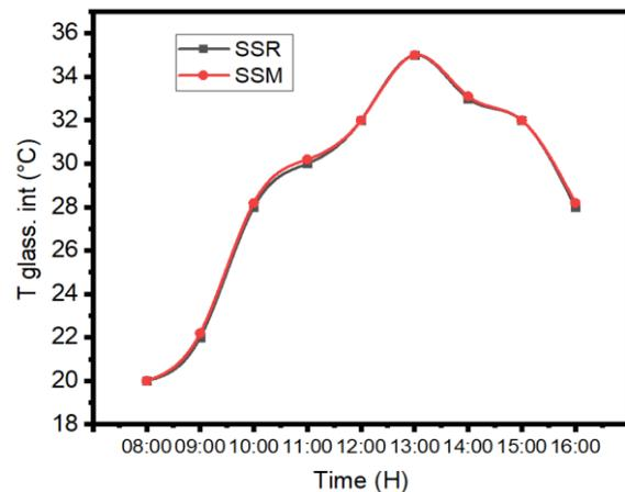
Figure 3. Evolution of internal glass cover temperature
