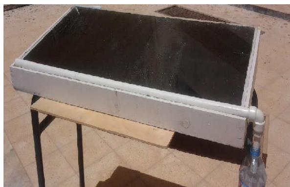
Figure 1. Single slope solar distiller
