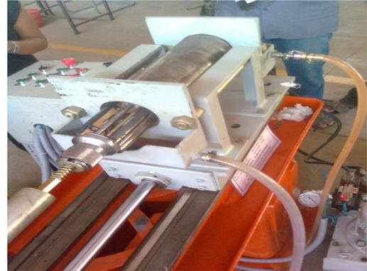
Figure 1 (b) Hydraulic sliding system
