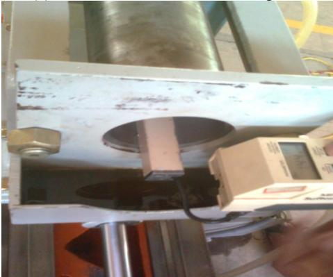
Figure 1 (c) Surface roughness measurement using Talysurf
