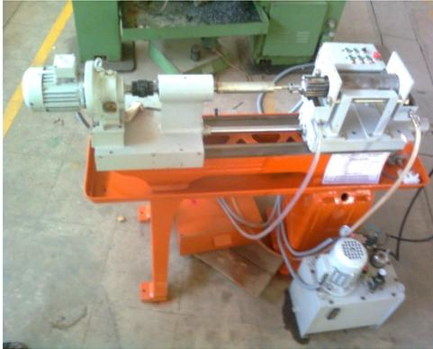
Figure 1(a) Retro fitted lathe with honing attachment
