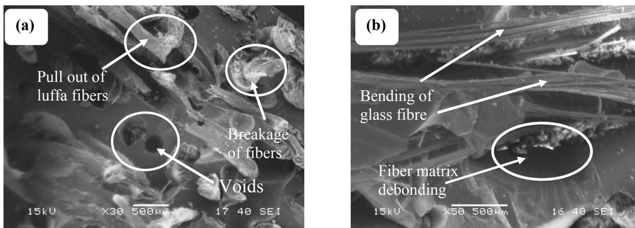
Figure 9. SEM image of fractured surface of laminates (a) S1 and (b) S5 under tensile load.
