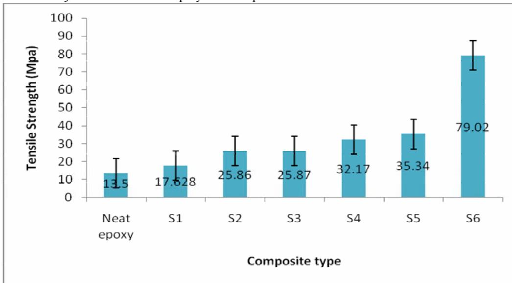
Figure 6. Tensile strength of the laminates.
