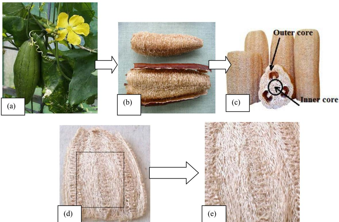
Figure 1. (a) The *luffa cylindrica* fruit (b) Dried *luffa* fruit with partial removed of outer layer (c) Sponge guard with hollow micro channels (d) Outer core open as mat (e) The rectangular portion used for making composite.
