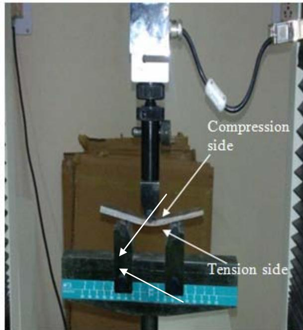
Figure 4. Three-point bending test with the specimen in loading position.
