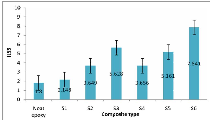
Figure 8. Interlaminar shear strength of the laminates.
