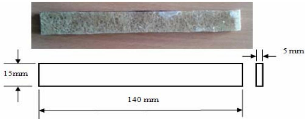
Figure 3. Flexural test configurations.
