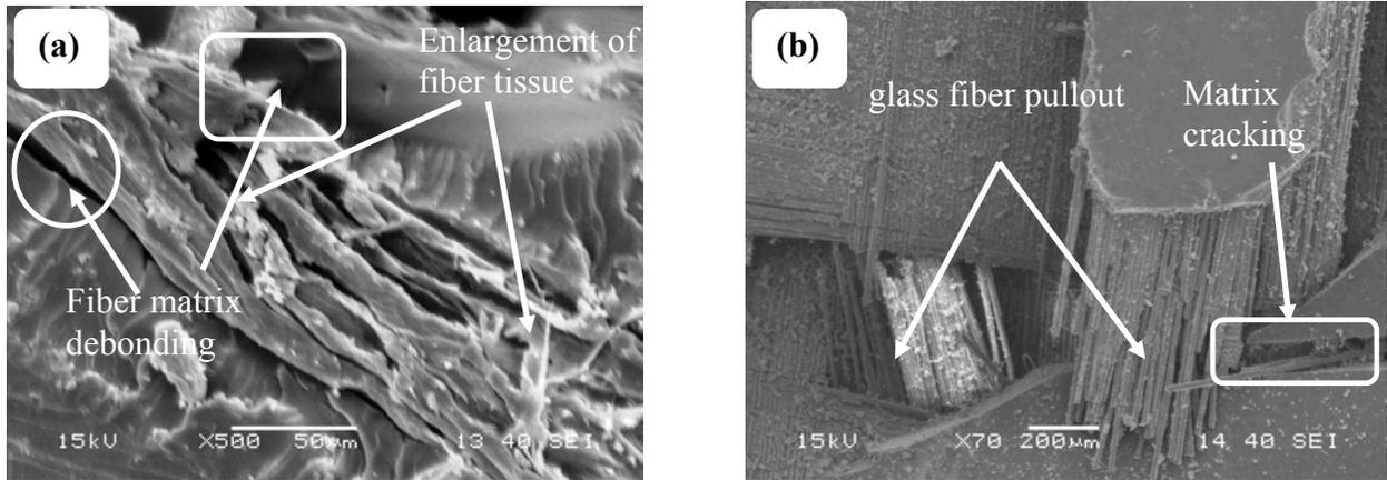
Figure 10. SEM image of tensile fractured surface of laminates (a) S1 and (b) S5 under flexural load.
