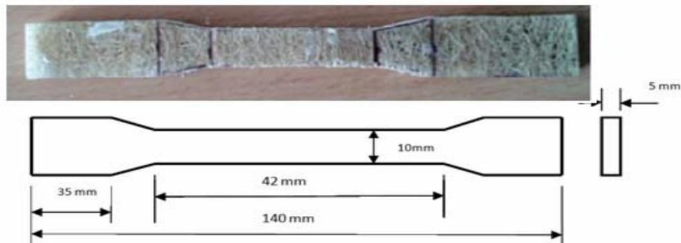
Figure 2. Tensile test configurations.
