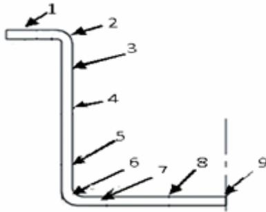
**Figure 3:** Measuring positions after cutting the drawing cups
