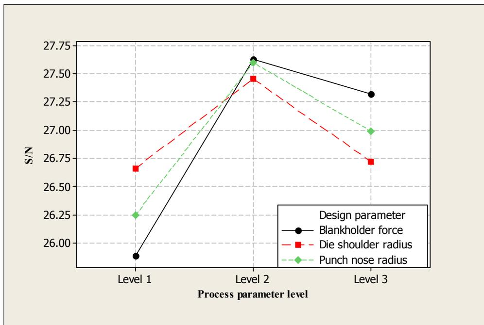
**Figure 6:** Plots of level average values of Punch nose radius die shoulder radius and blankholder force
