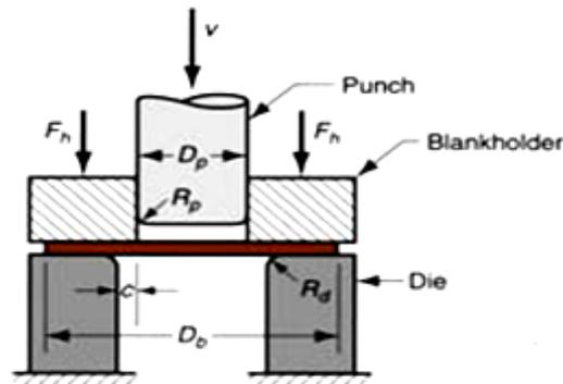
**Figure 2:** Scheme of deep drawing process (Patil and Bajaj, 2013)
