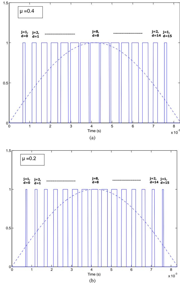
**Figure 6.** GWM based switching pulses with  $D=30$ , and  $f_m=60$  Hz for, (a)  $\mu=0.4$ , (b)  $\mu=0.2$ .
