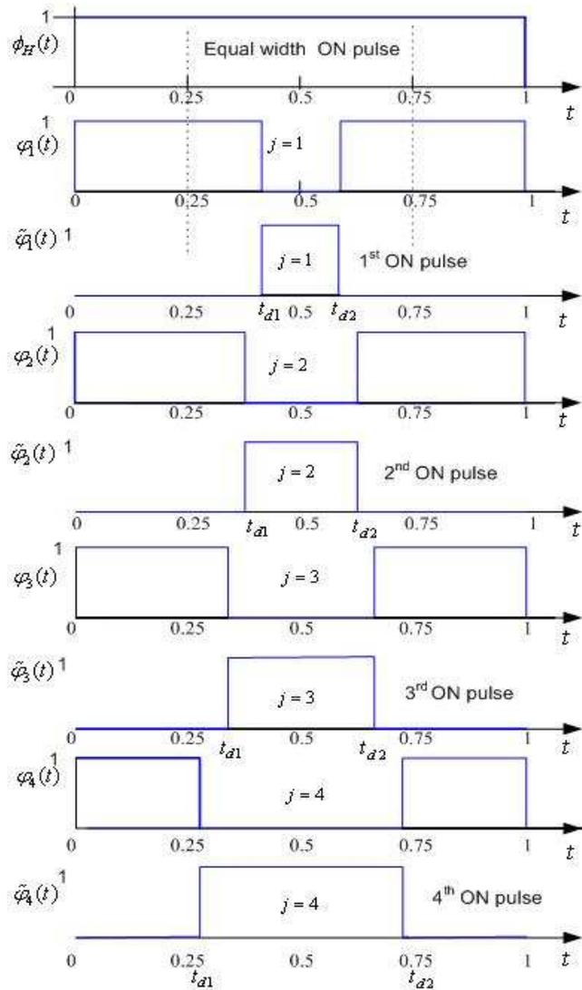
**Figure 5.** Variable width switching pulse generation using proposed method for  $\mu=0.2$  at normalized time scale.
