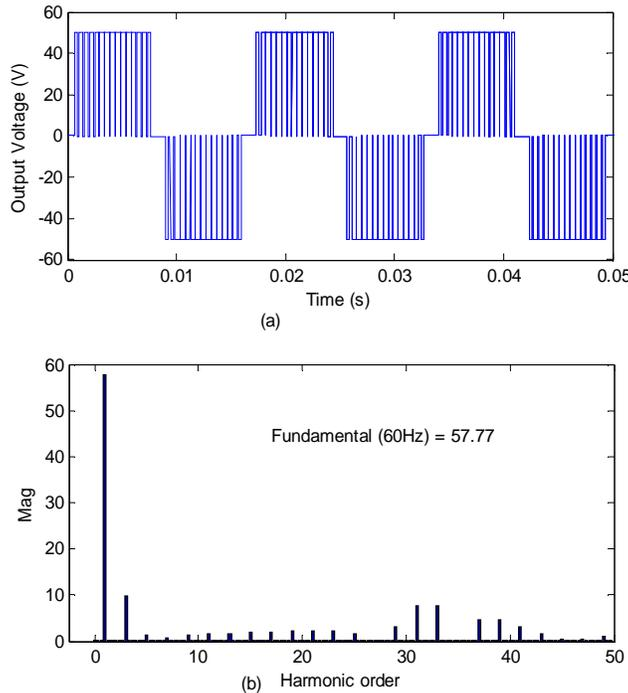
**Figure 4.** The switched dc-ac inverter output voltage due to basic wavelet modulation switching signals, (a) the output voltage, and (b) its spectrum
