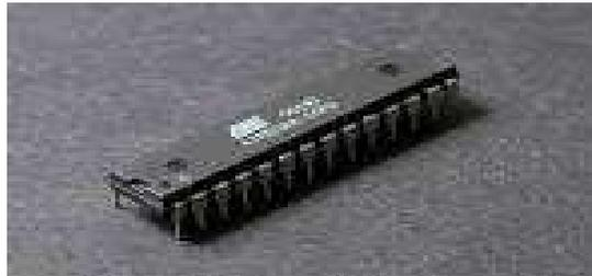
Figure 1. ATMEGA 8 Microcontroller
