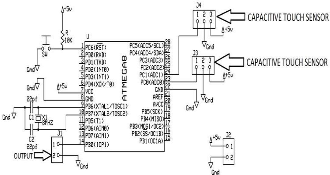
Figure 2. Hardware connection with ATMEGA 8
