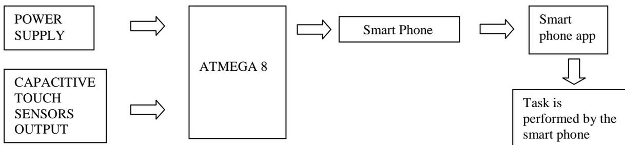
**Figure 11.** Showing Overall working of the Smart earphone
