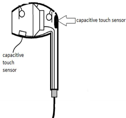
**Figure 9.** Showing both the sensors in one earphone lower one will touch the skin of the user when plugged in and the other one will not be touched by the skin when plugged in, it will be touched by the user finger.
