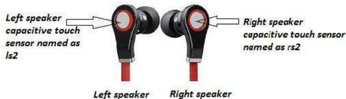
Figure 8. Back view of the Smart Earphone
