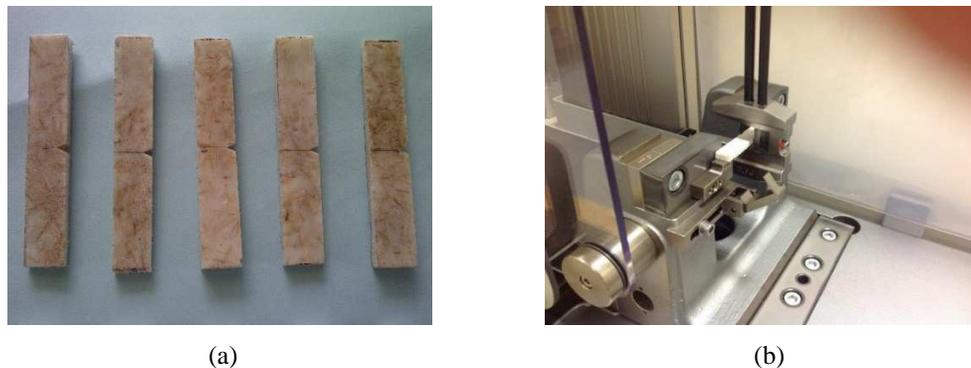
**Figure 1** (a) alkali-treated v-notched samples, and (b) edgewise impact blow configuration.
