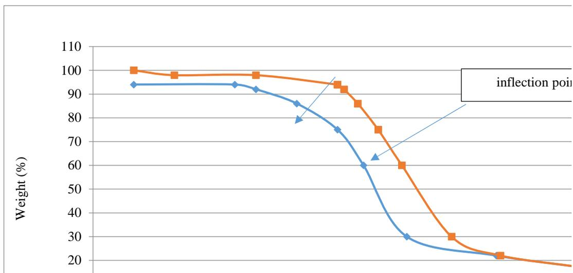
**Figure 3.** Reproduced TGA thermograms for untreated and alkali treated sisal fiber samples
