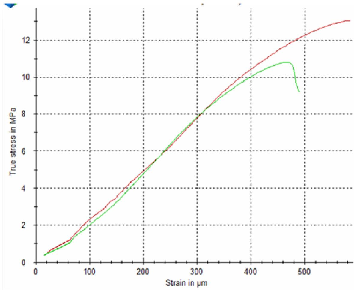
**Figure 5.** Tensile test curves for the two samples of the 25% NaOH treated fiber composites
