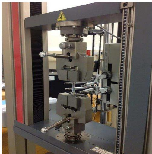
**Figure 2.** Zwick/Roell Z020 Universal testing machine illustrating sample positioning.
