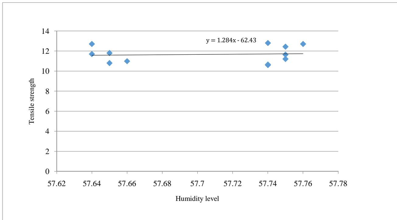
**Figure 7.** Variation in Tensile strength as a function of Humidity
