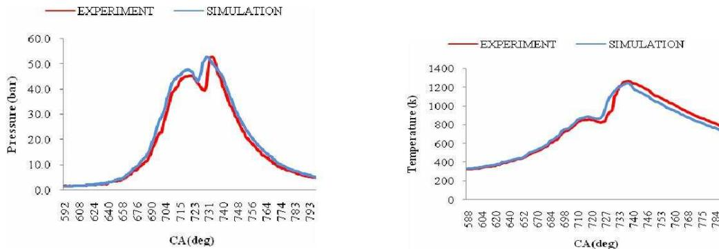
**Fig 4.** Comparison of cylinder pressure (bar) and temperature (K).
