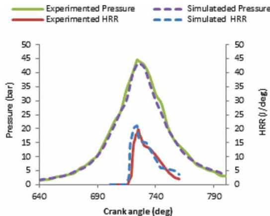
**Fig 5.** Comparison of cylinder pressure (bar) and heat release rate (J/deg).
