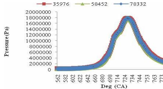
**Fig 2.** Grid independency test.
