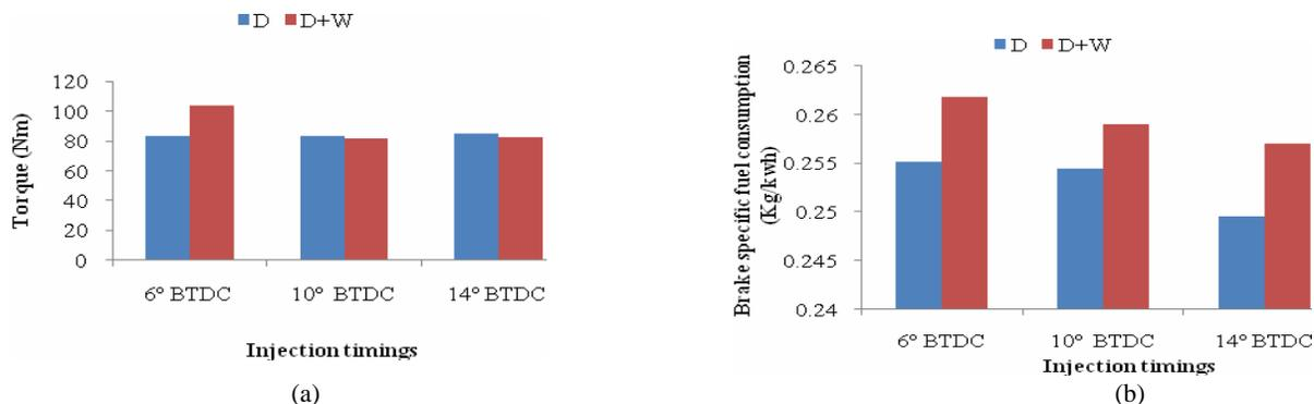
Fig 23. (a) Torque and (b) brake specific fuel consumptions at different injection timings
