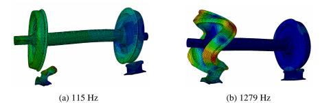
Figure 13. Flutter instability,  $K_x = K_y = 1000$  N/mm,  $K_z = 10000$  N/mm,  $\mu = 0.31$ .
