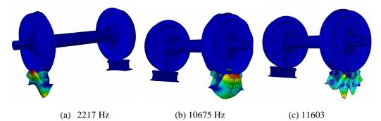
Figure 15. Flutter instability,  $K_x = K_y = 10^4$  N/mm,  $K_z = 10^8$  N/mm,  $\mu = 0.33, 0.35$ .
