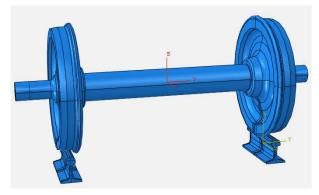
Figure 9. Finite element model of the wheelset and rails.
