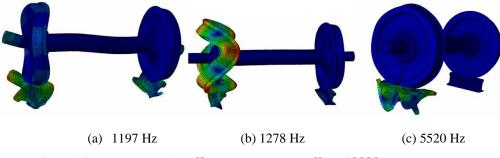
Figure 14. Flutter instability,  $K_x = K_y = 1000$  N/mm,  $K_z = 10000$  N/mm,  $\mu = 0.47$ .
