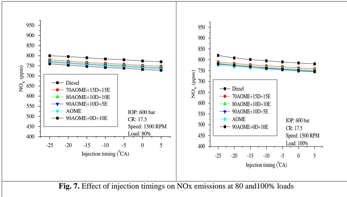
**Fig. 7.** Effect of injection timings on NO<sub>x</sub> emissions at 80 and 100% loads
