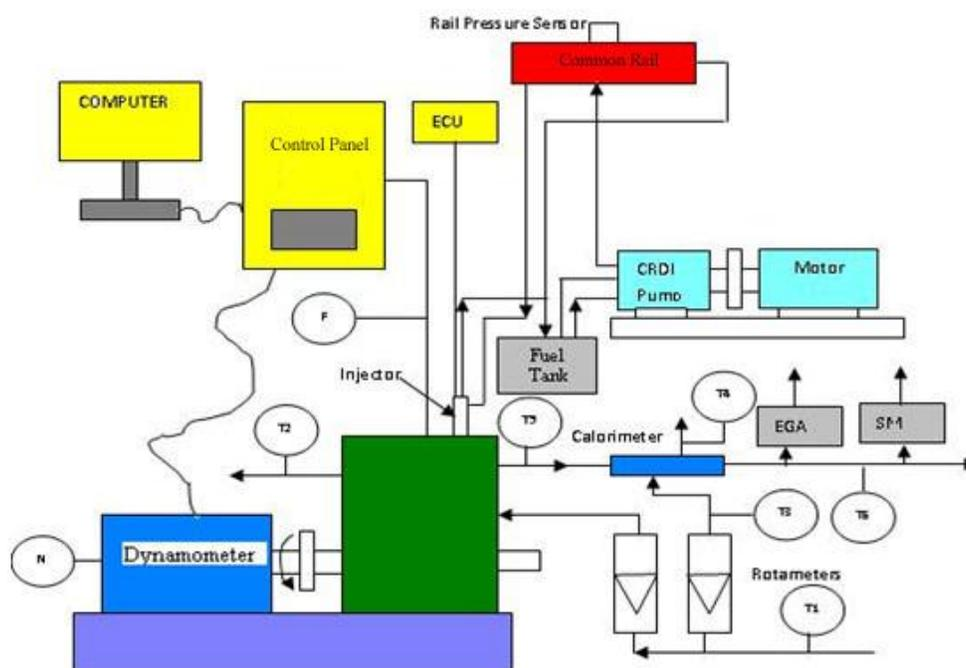
T1, T3 – Inlet Water Temperature, T2 – Outlet Engine Jacket Water Temperature
