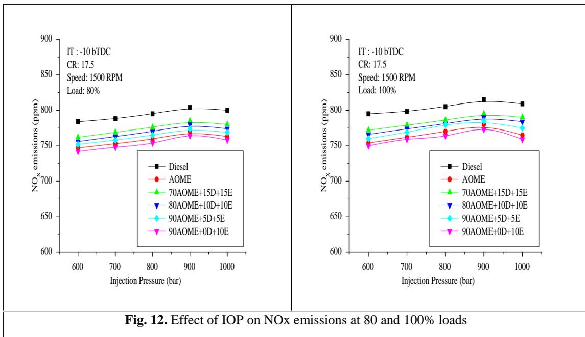
Fig. 12. Effect of IOP on NO<sub>x</sub> emissions at 80 and 100% loads
