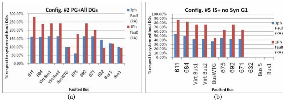
**Figure 2.** % of fault magnitude (3ph, 1ph) for all nodes respects to fault currents of system without DGs: (a) config. 2 (PG+ All DGs), (b) Config. 5 (IS+ All DGs-DG1)
