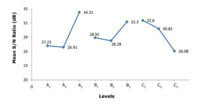
Figure 5 S/N ratio response graph for crystalline size
