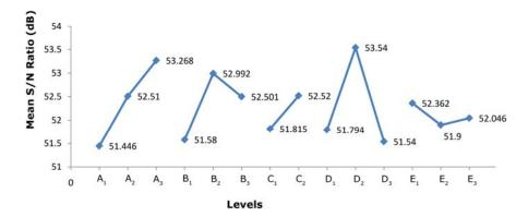
Figure 3 S/N ratio response graph for micro hardness (Legend: A: Rake angle; B: Depth of cut; C: Nose radius; D: Feed; E: Cutting velocity)
