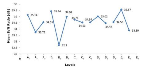
Figure 4 S/N ratio response graph for simultaneous optimization (Legend: A: Rake angle; B: Depth of cut; C: Nose radius; D: Feed; E: Cutting velocity)
