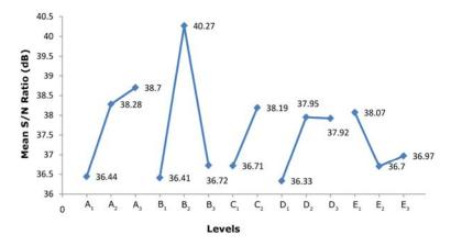
Figure 2 S/N ratio response graph for crystalline size
