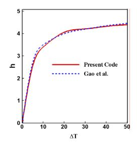
Fig. 3: Comparison between present code and Gao et al. (2000) at Pr = 0.73 and  $Ra = 10^4$
