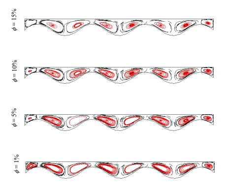
Fig. 8: Effect of  $\phi$  of water-CuO nanofluid on streamlines
