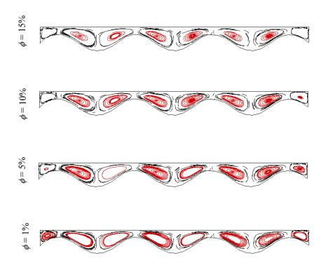
Fig. 6: Effect of  $\phi$  of water-Ag nanofluid on streamlines
