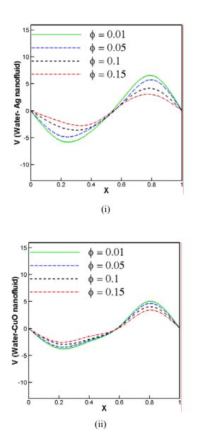
Fig. 14: Effect of volume fraction variation on the mid height vertical velocity (i) water-Ag nanofluid and (ii) water-CuO nanofluid
