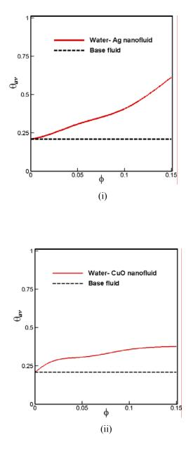
Fig. 11: Effect of volume fraction variation on the mean temperature of nanofluids (i) water-Ag nanofluid and (ii) water-CuO nanofluid
