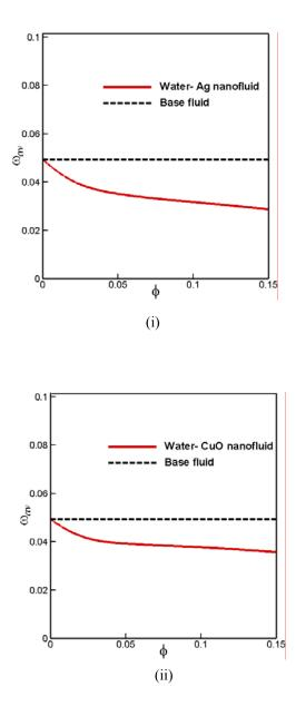
Fig. 12: Effect of volume fraction variation on the average velocity of nanofluids (i) water-Ag nanofluid and (ii) water-CuO nanofluid
