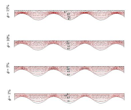
Fig. 5. Effect of  $\phi$  of water-Ag nanofluid on isothermal lines
