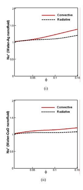
Fig. 10: Effect of volume fraction variation on the Nu\* (i) water-Ag nanofluid and (ii) water-CuO nanofluid
