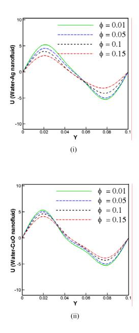
Fig. 13: Effect of volume fraction variation on the mid height horizontal velocity (i) water-Ag nanofluid and (ii) water-CuO nanofluid
