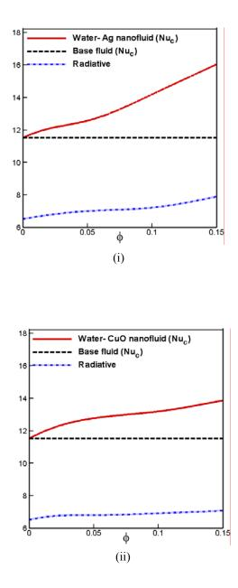
Fig. 9: Rate of heat transfer for the effect of  $\phi$  of (i) water-Ag nanofluid and (ii) water-CuO nanofluid
