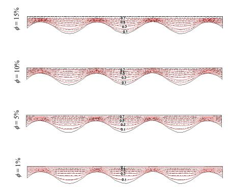
Fig. 7: Effect of  $\phi$  of water-CuO nanofluid on isothermal lines
