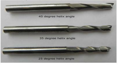
Fig. 1 Solid carbide end mill with different helix angles
