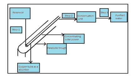
Figure 1. Flow diagram of set-up
