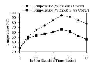
Figure 5. Temperature of fluid with glass cover and without glass cover
