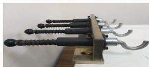
**Figure 5 :** Photograph of fixed hooks of machine, in which springs fitted assists movement of forward and backward movement to adjust for silk skein length shrinks during the Kilcha making process.
