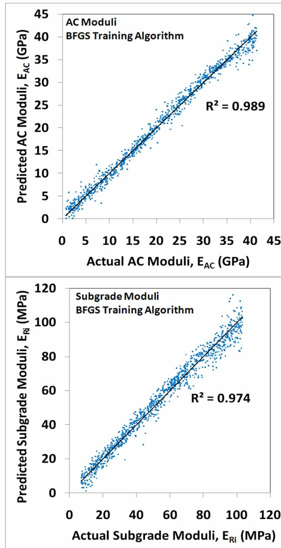
Figure 6. Neural networks AC and non-linear subgrade moduli prediction accuracies using BFGS training algorithm.
