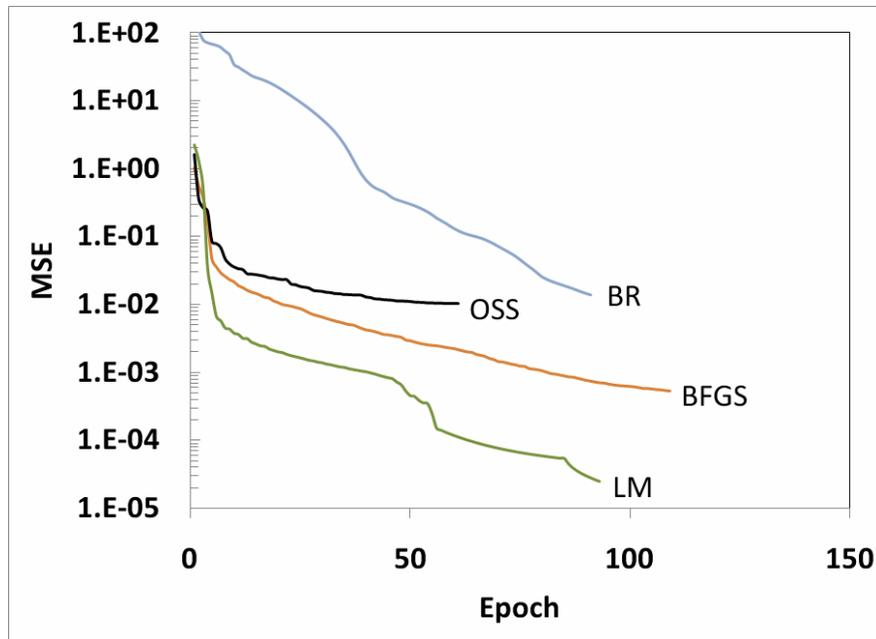
Figure 4. Effect of quasi-Newton and Levenberg-Marquardt backpropagation learning algorithms on training performance of FE-NN AC modulus prediction model
