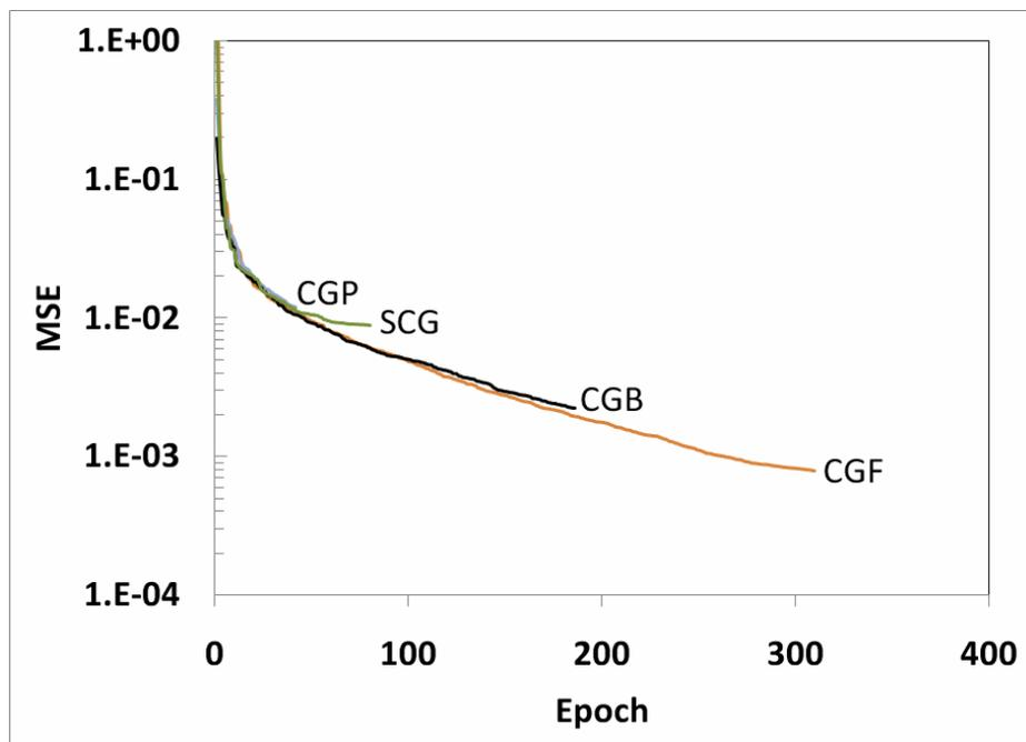
Figure 3. Effect of conjugate gradient backpropagation learning algorithms on training performance of FE-NN AC modulus prediction model
