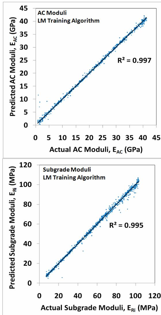
Figure 5. Neural networks AC and non-linear subgrade moduli prediction accuracies using Lavenberg-Marquardt (LM) training algorithm.
