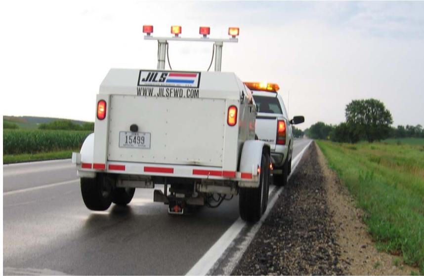
Figure 1. Non-destructive testing of pavements using Falling Weight Deflectometer (FWD)
