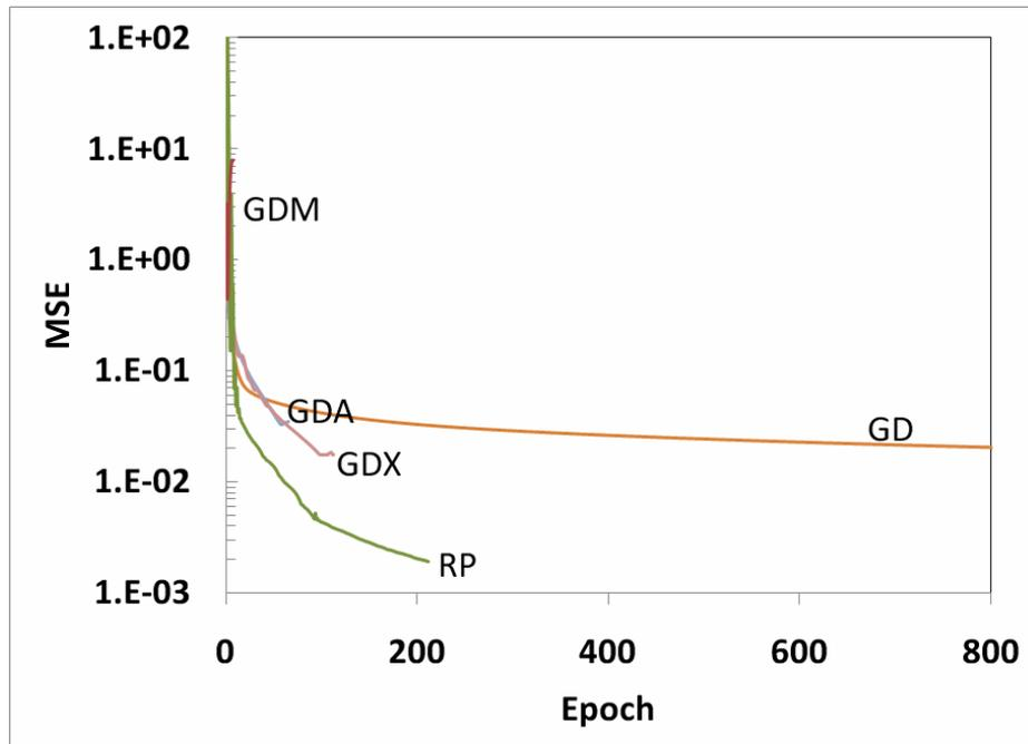
Figure 2. Effect of gradient-descent backpropagation learning algorithms on training performance of FE-NN AC modulus prediction model.
