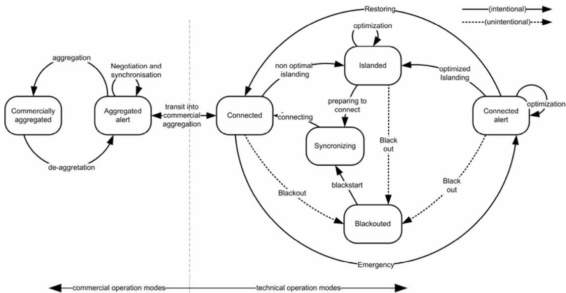
Figure 3. Control modes and transition for subgrid operation
