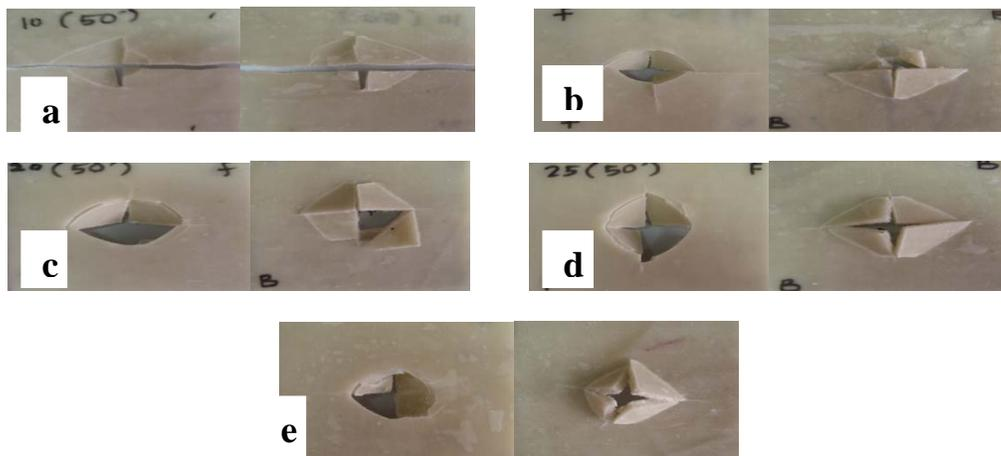
Figure 10. Specimens under 64J impact loading. (a) 10ply (b) 15ply (c) 20ply (d) 25ply (e) 30ply
