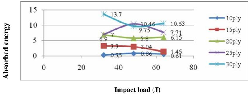
Figure 5. The absorption capability comparison of each composite category with increasing load
