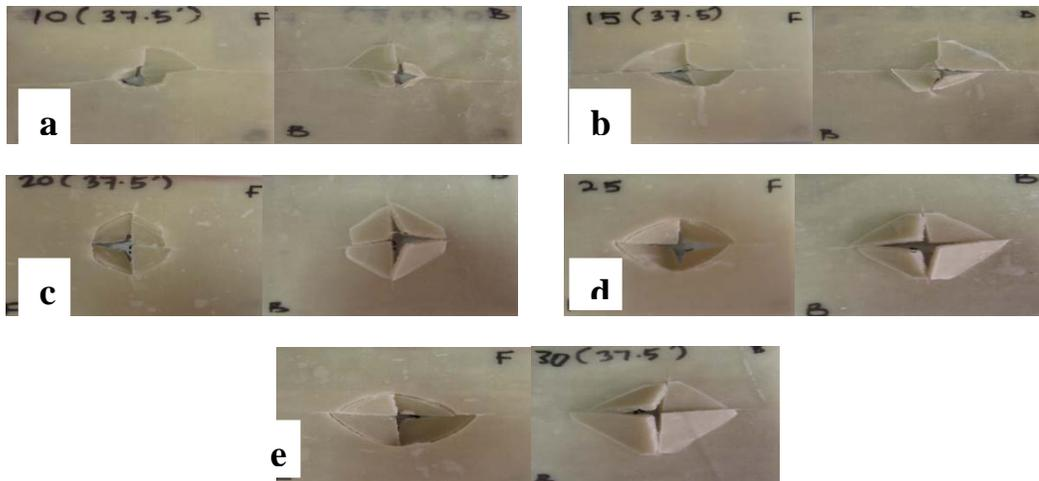
Figure 9. Specimens under 48J impact loading. (a) 10ply (b) 15ply (c) 20ply (d) 25ply (e) 30ply
