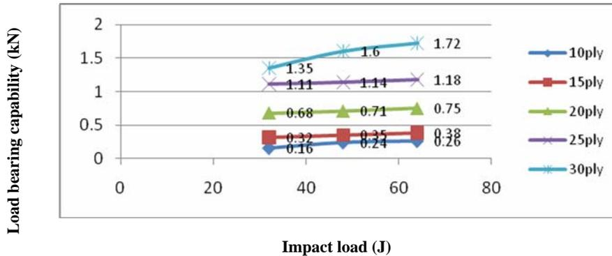
Figure 2. The effect of increasing load on the composite plates
