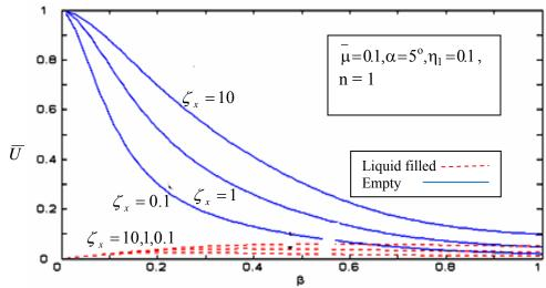
Figure 8. Axial displacement  $(\overline{U})$  vs. wave number  $(\beta)$  with stiffness coefficient  $\zeta_x = 0.1,1,10$  as parameter
