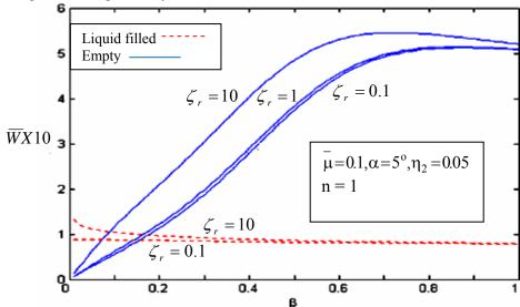
**Figure 1.** Radial displacement (W) vs. wave number ( $\beta$ ) with stiffness coefficient ( $\zeta_r$ ) as parameter
