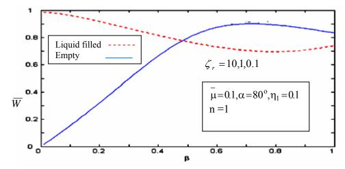
Figure 4. Radial displacement  $(\overline{W})$  vs. wave number  $(\beta)$  with damping coefficient  $\Gamma_r = 0.1,1,10$  as parameter
