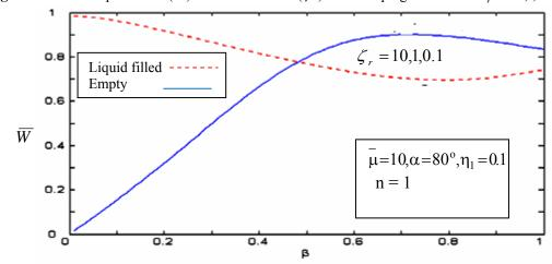
**Figure 6** Radial displacement ( $\overline{W}$ ) vs. wave number ( $\beta$ ) with  $\Gamma_r = 0.1,1,10$  as parameter
