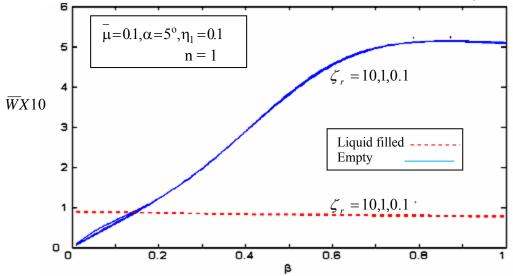
**Figure 2.** Radial displacement  $(\overline{W})$  vs. wave number  $(\beta)$  with stiffness coefficient  $\zeta_r = 0.1,1,10$  as parameter
