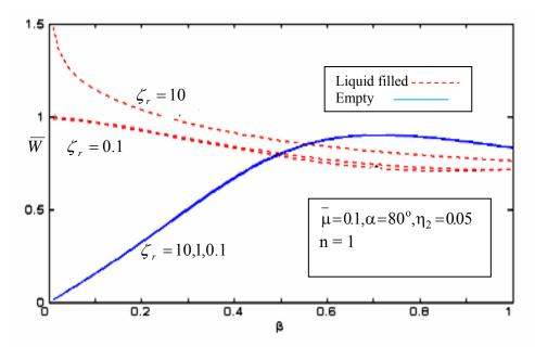
**Figure 3.** Radial displacement  $(\overline{W})$  vs. wave number  $(\beta)$  with stiffness  $\zeta_r = 0.1,1,10$  as parameter
