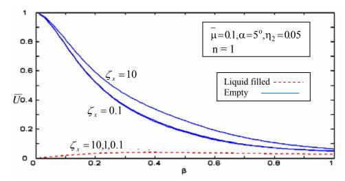
Figure 7. Axial displacement  $(\overline{U})$  vs. wave number  $(\beta)$  with stiffness coefficient  $\zeta_x = 0.1,1,10$  as parameter
