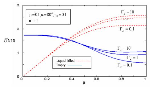
**Figure 10.** Axial displacement  $(\overline{U})$  vs. wave number  $(\beta)$  with damping coefficient  $\Gamma_x = 0.1,1,10$  as parameter
