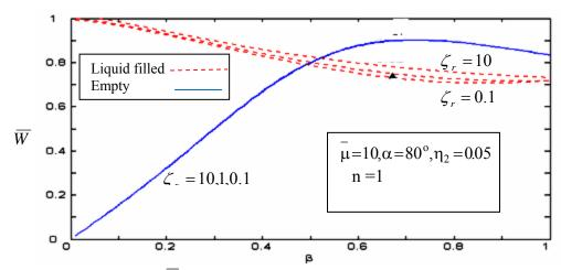
**Figure 5.** Radial displacement (W) vs. wave number ( $\beta$ ) with damping coefficient  $\Gamma_r = 0.1,1,10$  as parameter
