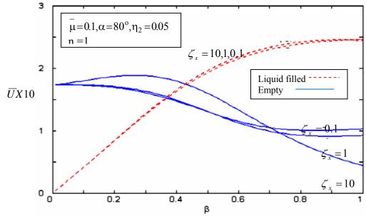
Figure 9. Axial displacement  $(\overline{U})$  vs. wave number  $(\beta)$  with stiffness coefficient  $\zeta_x = 0.1,1,10$  as parameter
