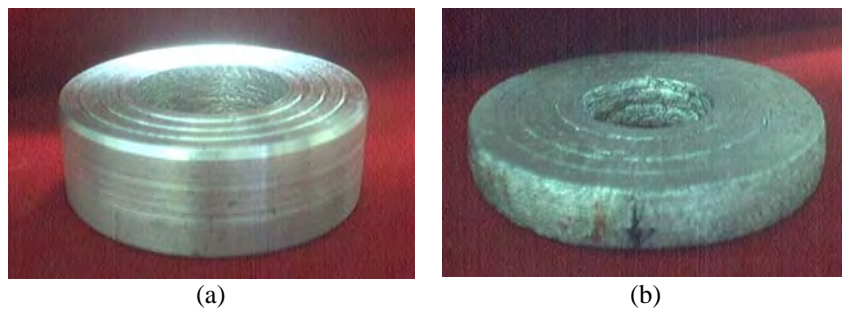
Figure 4 (b): Ring compression specimen (OD: ID: H = 6:3:2) (a) Undeformed (b) 50% deformed under dry condition (friction factor ‘m’=0.3).
