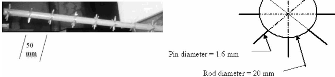
Figure 2. Rod-pin inserts (pin distance,  $x=50$  mm)
