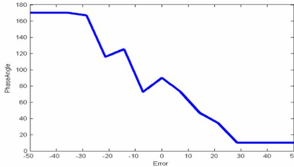
Figure 6. Defuzzified Output phase angle versus Input error
