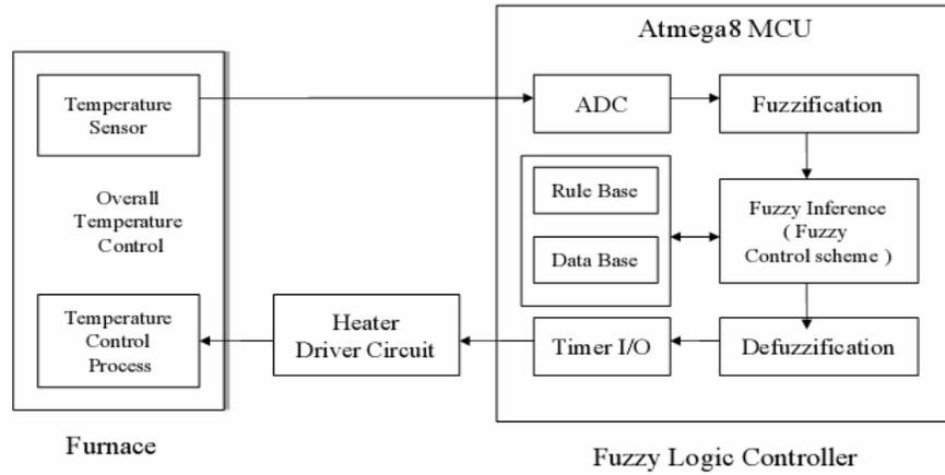
Figure 1. Block diagram of fuzzy logic temperature controller
