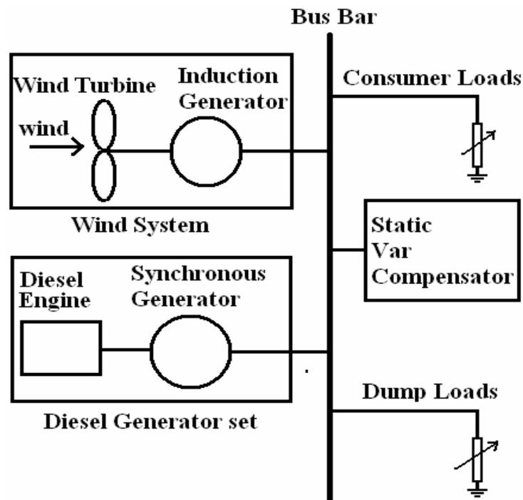
**Figure 1.** Block diagram of Autonomous Wind-Diesel Hybrid Power System
