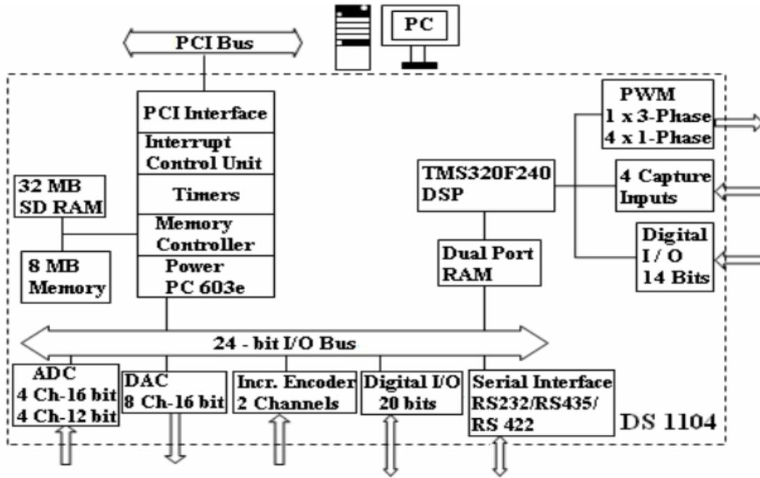
Figure 5. Block diagram of the DS 1104 controller board
