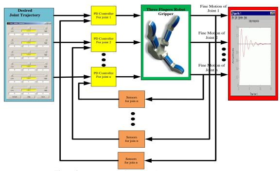
Figure 4 Control system of a n-DOF Fingers Robot Gripper
