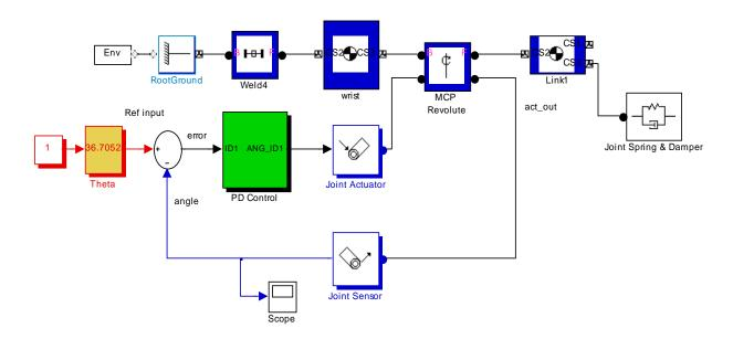
Figure 3 The abstraction of Physical modelling of MCP thumb gripper
