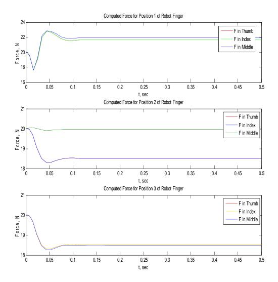
Figure 18 Simulation and control Force in the Position 1, 2, and 3 of Finger
