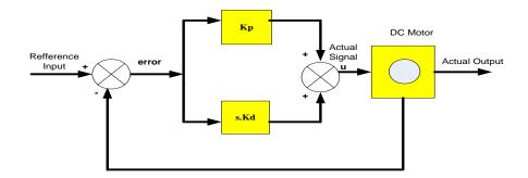
Figure 5 PD Control Diagram
