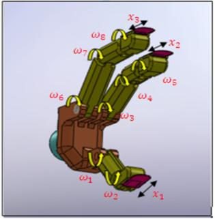
Figure 1. Architecture of Robot Gripper.
