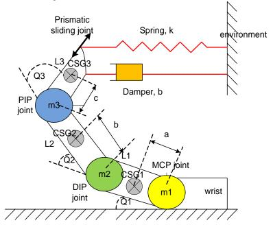
Figure 2 Finger model of robot hand.
