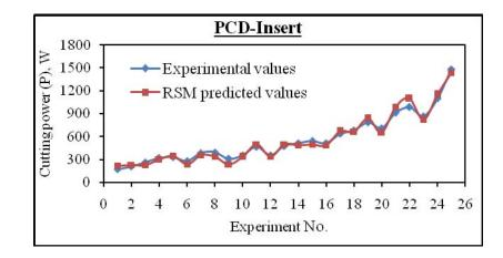
(c) Cutting power: Comparison between experimental values and RSM Predicted values for PCD insert.
