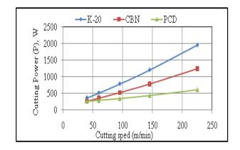
(a) Effect of cutting tool material on cutting Power with varying cutting speed on  $30^{\circ}$ Fiber orientation angle GFRP composite.
