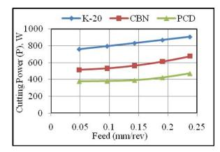
(c) Effect of cutting tool material on cutting power With varying feed on  $60^{\circ}$  fiber orientation angle GFRP composite.
