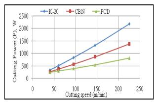
(e) Effect of cutting tool materail on cutting power With varying cutting speed on 90<sup>0</sup> fiber orientation Angle GFRP composite.
