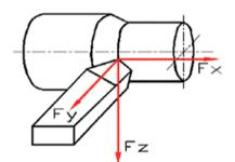
Figure 2: Details of the force measurement
