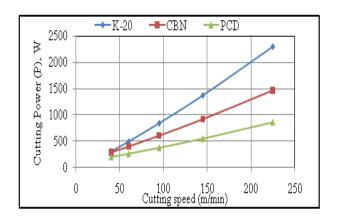
(d) Effect of cutting tool material on cutting power with varying cutting speed on 75<sup>o</sup> fiber orientation GFRP composite.
