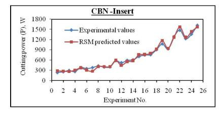
(b) Cutting power: Comparison between experimental values and RSM Predicted values for CBN insert.
