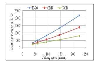
(c) Effect of cutting tool material on cutting Power with varying cutting speed on  $60^{\circ}$ fiber orientation angle GFRP composite.
