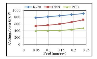
(d) Effect of cutting tool material on cutting power with varying feed on  $75^0$  fiber orientation angle GFRP composite.
