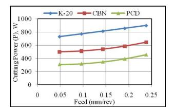
(b) Effect of cutting tool material on cutting power with varying feed on  $45^0$  fiber orientation angle GFRP composite.
