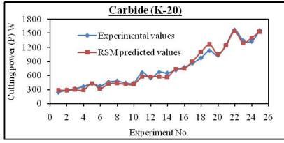
(a) Cutting power: Comparison between experimental values and RSM Predicted values for Carbide-(K-20) insert.
