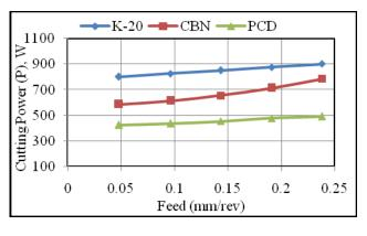
(e) Effect of cutting tool material on cutting power With varying feed on 90<sup>0</sup> fiber orientation angle GFRP composite.
