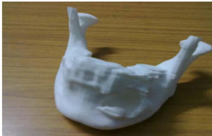
**Figure 6:** RP model of 0.6mm layer thickness and 0.3 mm interval thickness
