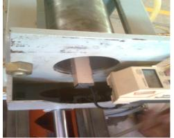
Figure 1 (c) Surface roughness measurement using Talysurf Figure 1: Experimental set up
