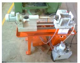
Figure 1(a) Retro fitted lathe with honing attachment
