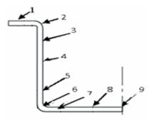
Figure 3: Measuring positions after cutting the drawing cups
