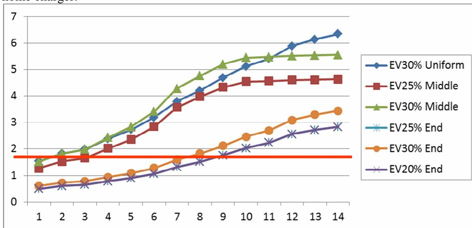
Figure 9. % VU vs. Time (h) with PEVs connected location in V2G mode
