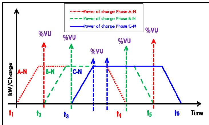
Fig. 2. Model of PEVs charging and discharging behavior on the distribution system
