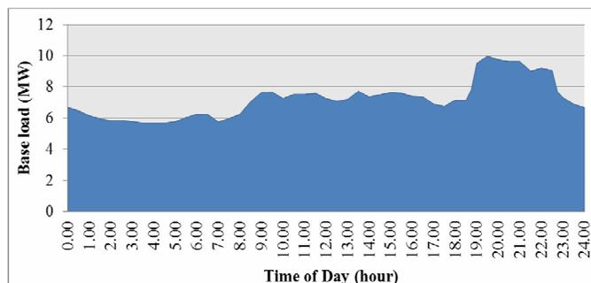
Figure A.1. Daily load profile of Feeder 9, Nakhon Sawan-2 substation
