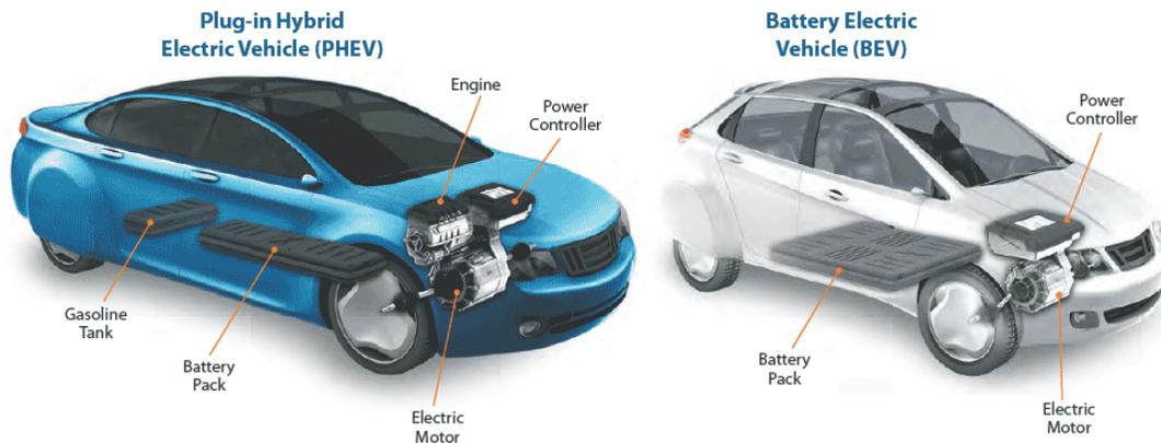
**Figure 1.** System technology of PEV
