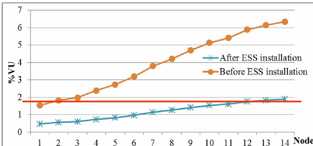
Figure 19. Voltage unbalance in V2G mode before and after ESS installation
