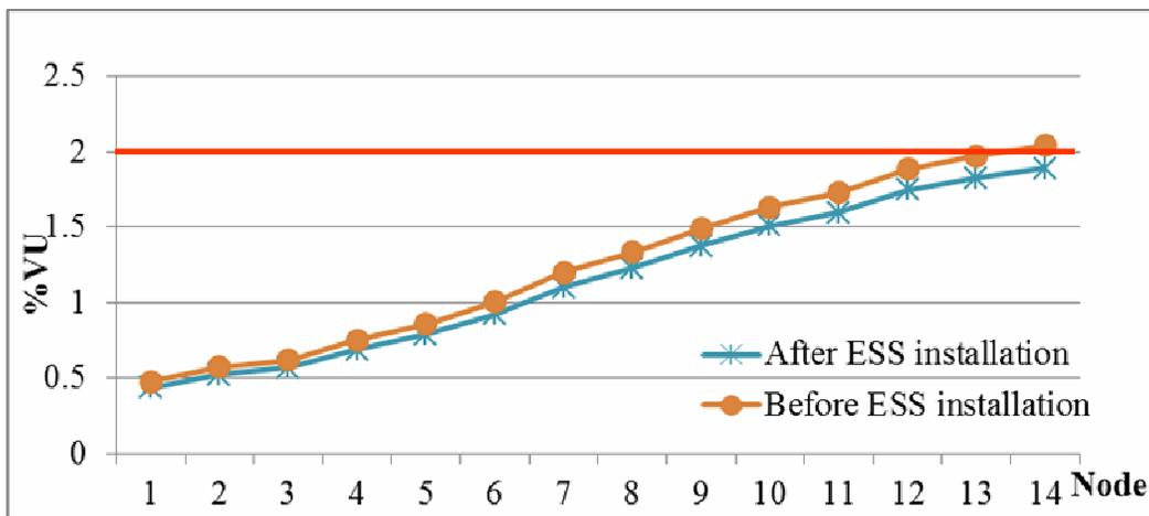
Figure 18. Voltage unbalance in G2V mode before and after ESS installation
