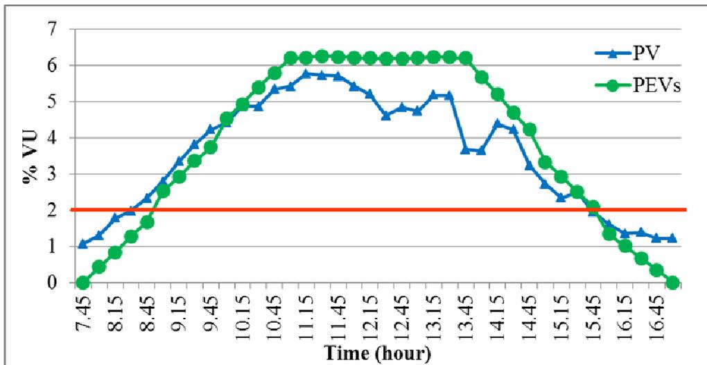
Figure 14. Voltage unbalance comparison between PV and PEVs
