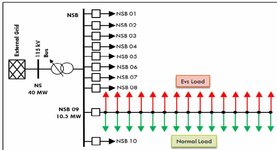
Figure 3. Configuration of the test system
