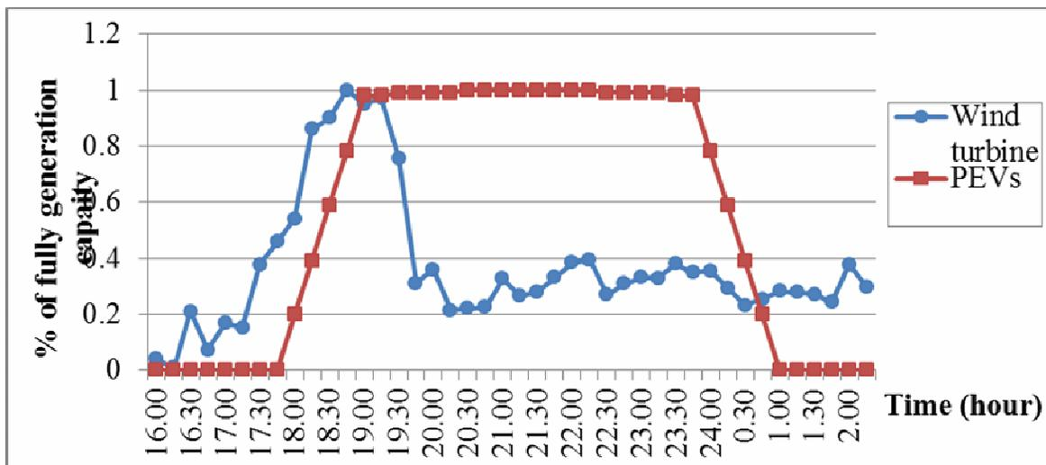
Figure 13. Wind turbine and PEVs daily generation shape comparison
