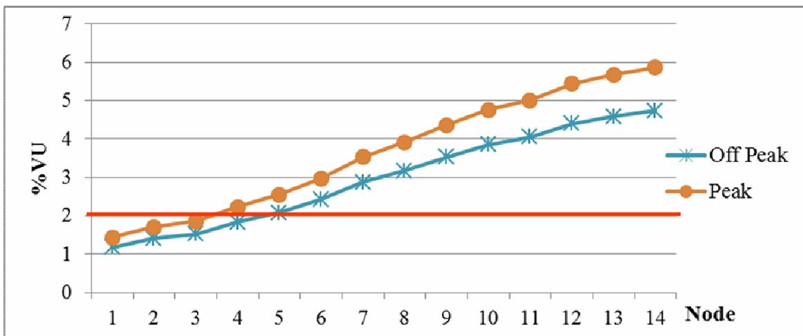
Figure 17. Voltage unbalance mitigation by generation shift due to TOU rate
