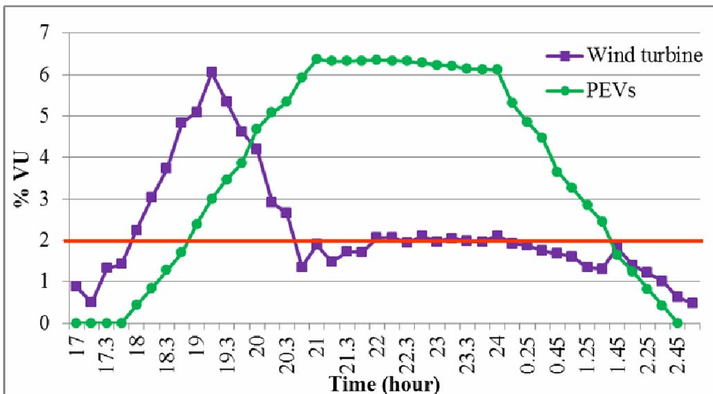
Figure 15. Voltage unbalance comparison between Wind turbine and PEVs
