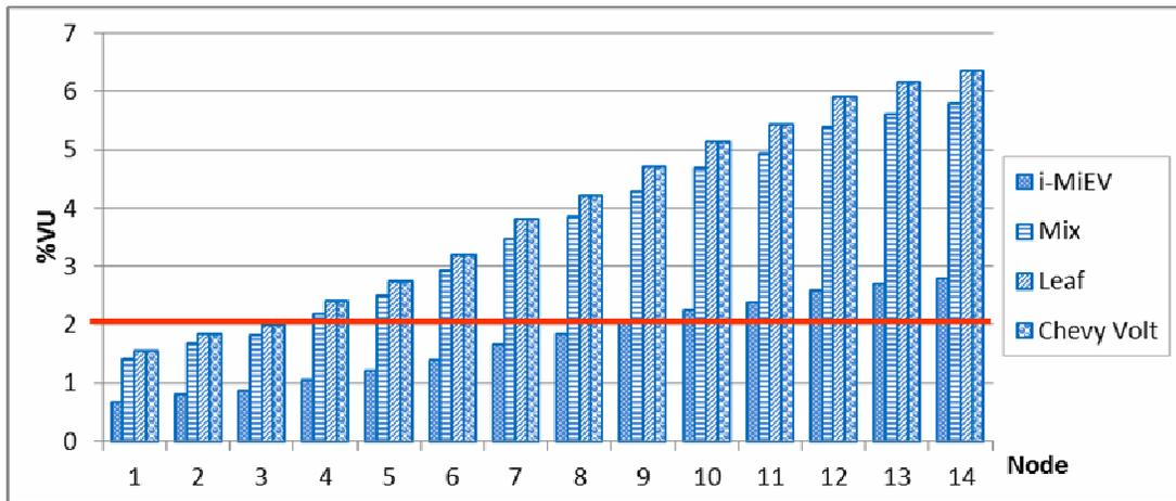
Figure 10. %VU vs. Time (h) with different PEVs charging rate in V2G mode
