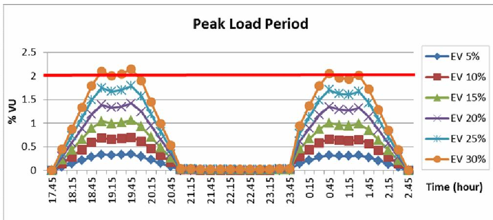
**Figure 4.** % VU vs. Time (h) with different PEVs penetration levels in G2V mode
