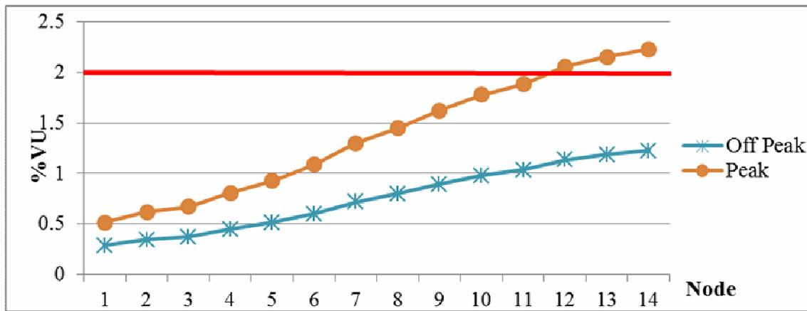
Figure 16. Voltage unbalance mitigation by load shift due to TOU rate
