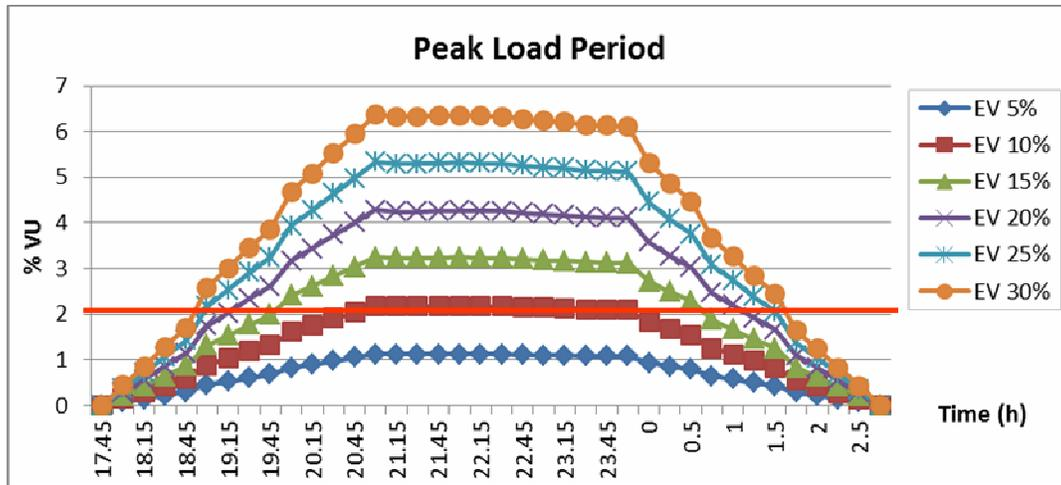
Figure 8. % VU vs. Time (h) with different PEVs penetration levels in V2G mode
