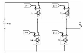
Figure 1. Single phase four pulse H-bridge inverter
