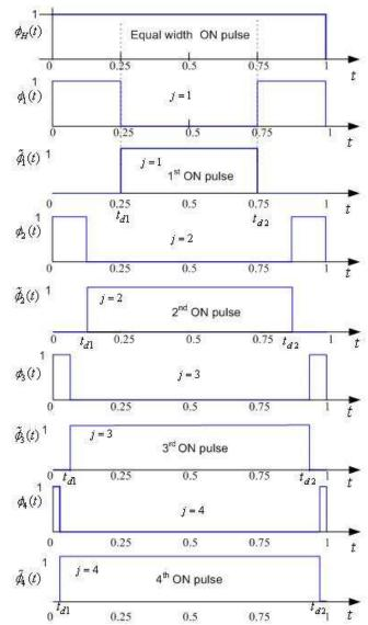
In order to represent a signal at different resolution levels, the used scaling function must be dilated (scaled) and translated (shifted).
