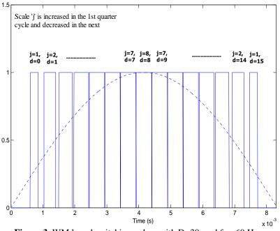
Figure 3. WM based switching pulses with D=30, and fm=60 Hz
