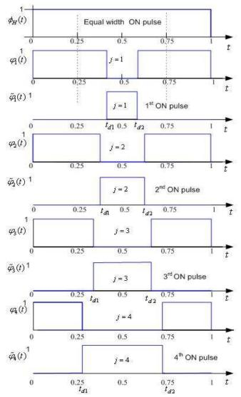
**Figure 5.** Variable width switching pulse generation using proposed method for  $\mu$ =0.2 at normalized time scale.
