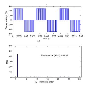
Figure 7. The switched dc-ac inverter output voltage due to generalized wavelet modulation switching signals for D=30 and  $\mu$ =0.4, (a) the output voltage and (b) its spectrum
